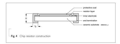
resistance value. Finally, the two external terminations (pure Tin) are added. See fig. 4.
